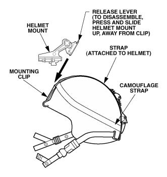
Figure 2-19. Attaching the Helmet Mount to the Strap.
